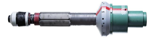
Our **CRTi tools** are designed for casing running or drilling with top drive equipped rigs to enable connection makeup, break-out, circulation and rotation, increasing the chance of getting casing to TD the first time. These tools are mechanically activated in tension and both rotational directions solely by top drive control using TAWG™ (Torque activated Wedge grip) technology.
